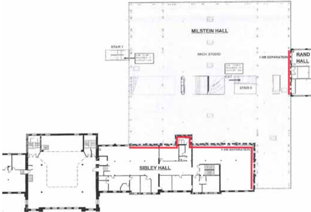
Figure 5. Fire separation shown at the upper level of Milstein Hall (red lines have been added by J. Ochshorn to match what appeared in the original colored drawings, prepared by KHA Architects, dated 5/5/09).
